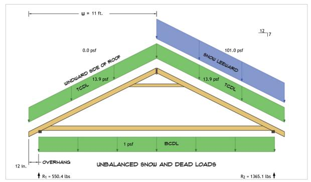
$R_1 = D + S = 217.1 \text{ lbs} + 333.3 \text{ lbs}$  $R_2 = D + S = 217.1 \text{ lbs} + 1148.0 \text{ lbs}$
