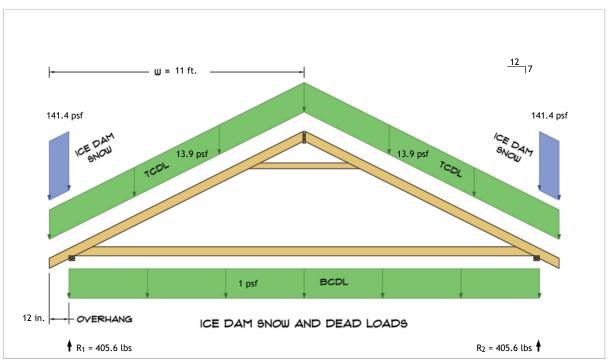
$R_1 = D + S = 217.1 \text{ lbs} + 188.5 \text{ lbs}$  $R_2 = D + S = 217.1 \text{ lbs} + 188.5 \text{ lbs}$
