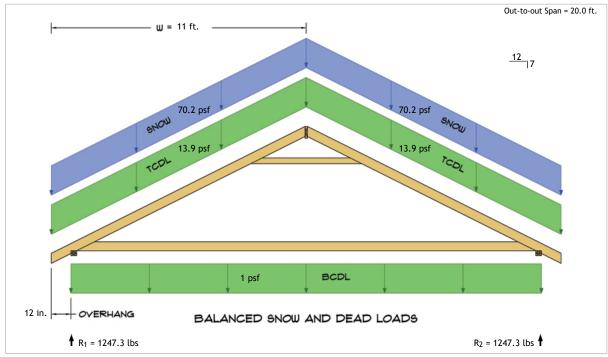
$R_1 = D + S = 217.1 \text{ lbs} + 1030.2 \text{ lbs}$  $R_2 = D + S = 217.1 \text{ lbs} + 1030.2 \text{ lbs}$
