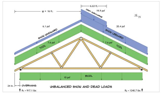
$R_1 = D + S = 522.7 \text{ lbs} + 394.4 \text{ lbs}$  $R_2 = D + S = 522.7 \text{ lbs} + 718.0 \text{ lbs}$
