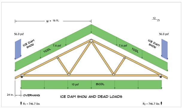
$$\begin{split} R_1 &= D + S = 522.7 \text{ lbs} + 224.0 \text{ lbs} \\ R_2 &= D + S = 522.7 \text{ lbs} + 224.0 \text{ lbs} \end{split}$$
