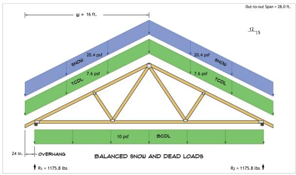
$\begin{aligned} R_1 &= D + S = 522.7 \text{ lbs} + 653.1 \text{ lbs} \\ R_2 &= D + S = 522.7 \text{ lbs} + 653.1 \text{ lbs} \end{aligned}$
