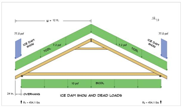
$$\begin{split} R_1 &= D + S = 248.8 \text{ lbs} + 205.3 \text{ lbs} \\ R_2 &= D + S = 248.8 \text{ lbs} + 205.3 \text{ lbs} \end{split}$$
