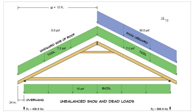
$R_1 = D + S = 248.8 \text{ lbs} + 160.0 \text{ lbs}$  $R_2 = D + S = 248.8 \text{ lbs} + 640.0 \text{ lbs}$
