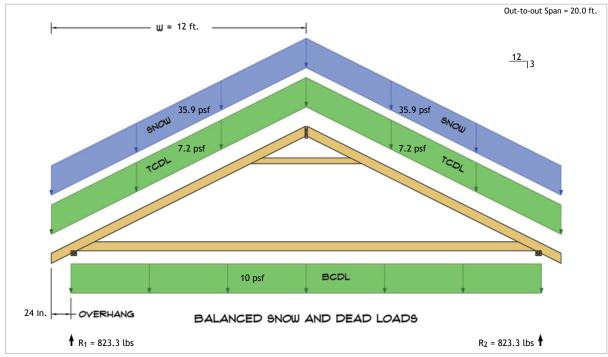
$R_1 = D + S = 248.8 \text{ lbs} + 574.5 \text{ lbs}$  $R_2 = D + S = 248.8 \text{ lbs} + 574.5 \text{ lbs}$
