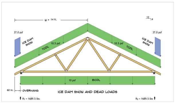
$\begin{aligned} R_1 &= D + S = 950.3 \text{ lbs} + 739.2 \text{ lbs} \\ R_2 &= D + S = 950.3 \text{ lbs} + 739.2 \text{ lbs} \end{aligned}$
