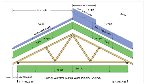
$R_1 = D + S = 950.3 \text{ lbs} + 460.3 \text{ lbs}$  $R_2 = D + S = 950.3 \text{ lbs} + 1089.4 \text{ lbs}$
