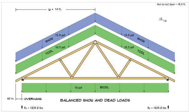
$\begin{aligned} R_1 &= D + S = 950.3 \text{ lbs} + 889.5 \text{ lbs} \\ R_2 &= D + S = 950.3 \text{ lbs} + 889.5 \text{ lbs} \end{aligned}$
