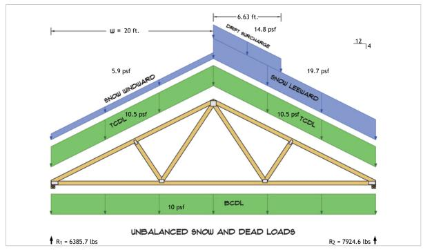
$R_1 = D + S = 4108.2 \text{ lbs} + 2277.5 \text{ lbs}$  $R_2 = D + S = 4108.2 \text{ lbs} + 3816.4 \text{ lbs}$
