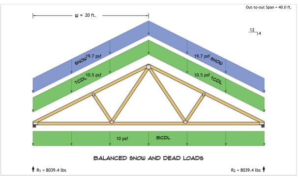
$R_1 = D + S = 4108.2 \text{ lbs} + 3931.2 \text{ lbs}$  $R_2 = D + S = 4108.2 \text{ lbs} + 3931.2 \text{ lbs}$
