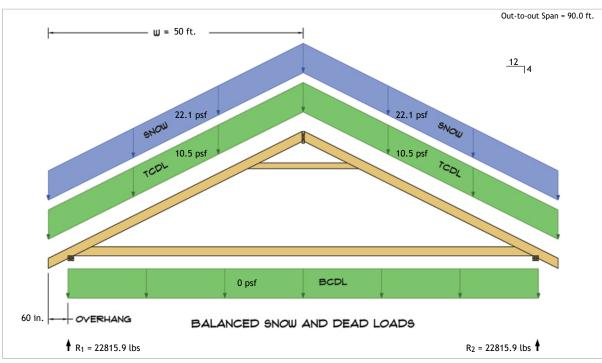
$$\begin{split} R_1 &= D + S = 7378.6 \text{ lbs} + 15437.2 \text{ lbs} \\ R_2 &= D + S = 7378.6 \text{ lbs} + 15437.2 \text{ lbs} \end{split}$$
