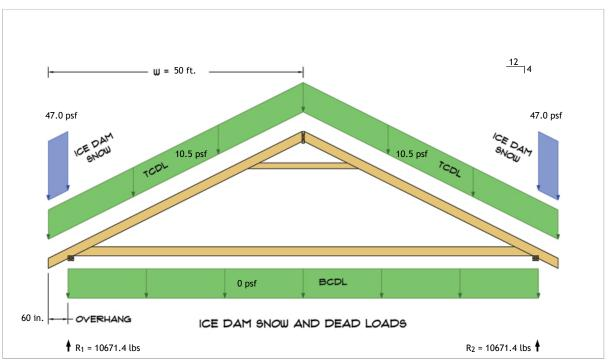
$R_1 = D + S = 7378.6 \text{ lbs} + 3292.8 \text{ lbs}$  $R_2 = D + S = 7378.6 \text{ lbs} + 3292.8 \text{ lbs}$
