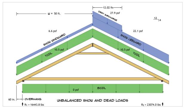
$R_1 = D + S = 7378.6 \text{ lbs} + 9065.2 \text{ lbs}$  $R_2 = D + S = 7378.6 \text{ lbs} + 15695.3 \text{ lbs}$
