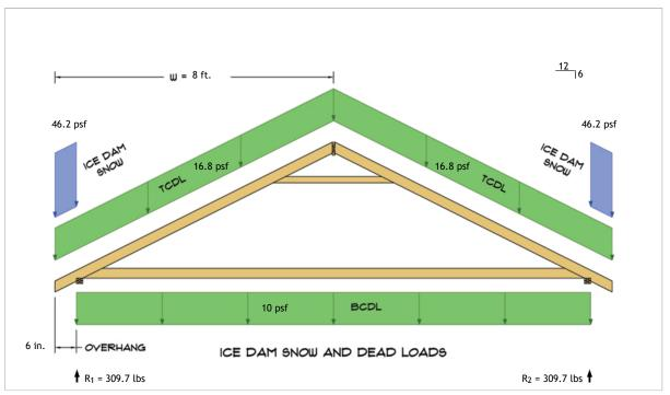
$$\begin{split} R_1 &= D + S = 278.9 \text{ lbs} + 30.8 \text{ lbs} \\ R_2 &= D + S = 278.9 \text{ lbs} + 30.8 \text{ lbs} \end{split}$$
