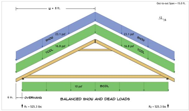
$R_1 = D + S = 278.9 \text{ lbs} + 246.4 \text{ lbs}$  $R_2 = D + S = 278.9 \text{ lbs} + 246.4 \text{ lbs}$
