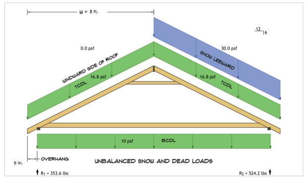
$R_1 = D + S = 278.9 \text{ lbs} + 74.7 \text{ lbs}$  $R_2 = D + S = 278.9 \text{ lbs} + 245.3 \text{ lbs}$
