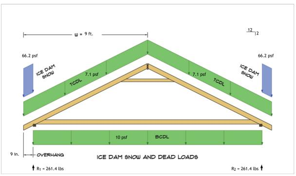
$$\begin{split} R_1 &= D + S = 195.2 \text{ lbs} + 66.2 \text{ lbs} \\ R_2 &= D + S = 195.2 \text{ lbs} + 66.2 \text{ lbs} \end{split}$$
