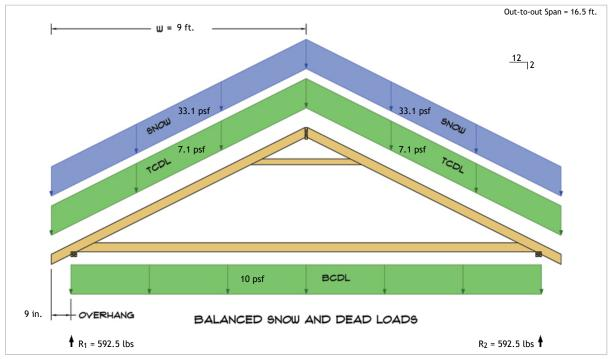
$R_1 = D + S = 195.2 \text{ lbs} + 397.3 \text{ lbs}$  $R_2 = D + S = 195.2 \text{ lbs} + 397.3 \text{ lbs}$
