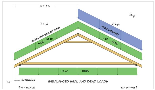
$R_1 = D + S = 195.2 \text{ lbs} + 117.3 \text{ lbs}$  $R_2 = D + S = 195.2 \text{ lbs} + 398.7 \text{ lbs}$
