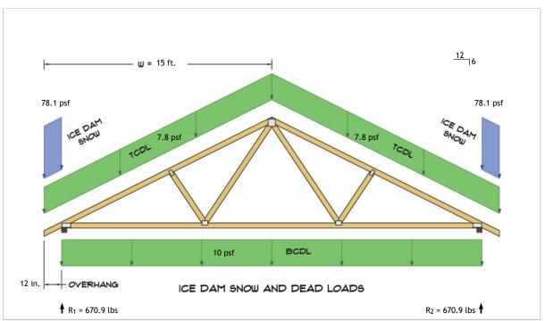
$R_1 = D + S = 514.8 \text{ lbs} + 156.2 \text{ lbs}$  $R_2 = D + S = 514.8 \text{ lbs} + 156.2 \text{ lbs}$
