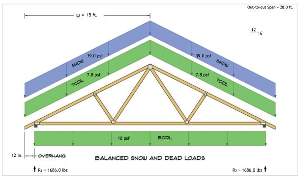
$\begin{aligned} R_1 &= D + S = 514.8 \text{ lbs} + 1171.2 \text{ lbs} \\ R_2 &= D + S = 514.8 \text{ lbs} + 1171.2 \text{ lbs} \end{aligned}$
