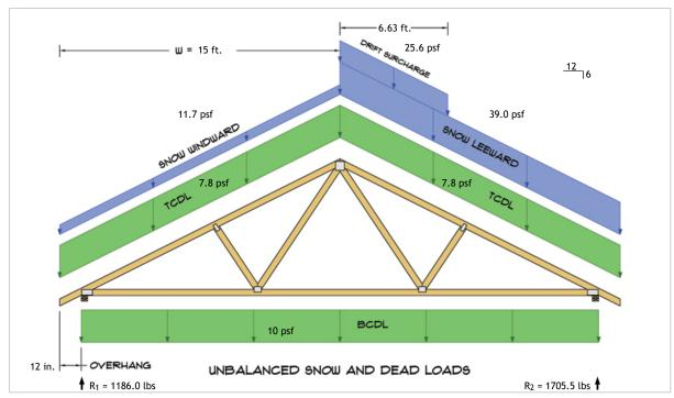
$R_1 = D + S = 514.8 \text{ lbs} + 671.2 \text{ lbs}$  $R_2 = D + S = 514.8 \text{ lbs} + 1190.7 \text{ lbs}$
