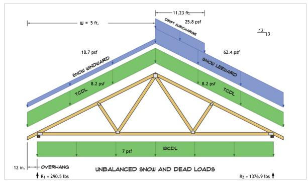
$R_1 = D + S = 138.5 \text{ lbs} + 152.1 \text{ lbs}$  $R_2 = D + S = 138.5 \text{ lbs} + 1238.4 \text{ lbs}$
