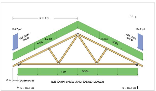
$R_1 = D + S = 138.5 \text{ lbs} + 249.5 \text{ lbs}$  $R_2 = D + S = 138.5 \text{ lbs} + 249.5 \text{ lbs}$
