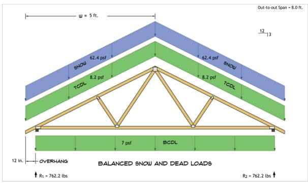
$$\begin{split} R_1 &= D + S = 138.5 \text{ lbs} + 623.7 \text{ lbs} \\ R_2 &= D + S = 138.5 \text{ lbs} + 623.7 \text{ lbs} \end{split}$$
