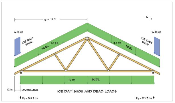
$\begin{aligned} R_1 &= D + S = 679.7 \text{ lbs} + 184.0 \text{ lbs} \\ R_2 &= D + S = 679.7 \text{ lbs} + 184.0 \text{ lbs} \end{aligned}$
