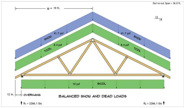
$R_1 = D + S = 679.7 \text{ lbs} + 1586.4 \text{ lbs}$  $R_2 = D + S = 679.7 \text{ lbs} + 1586.4 \text{ lbs}$
