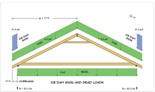
$R_1 = D + S = 0.0 \text{ lbs} + 83.2 \text{ lbs}$  $R_2 = D + S = 0.0 \text{ lbs} + 83.2 \text{ lbs}$
