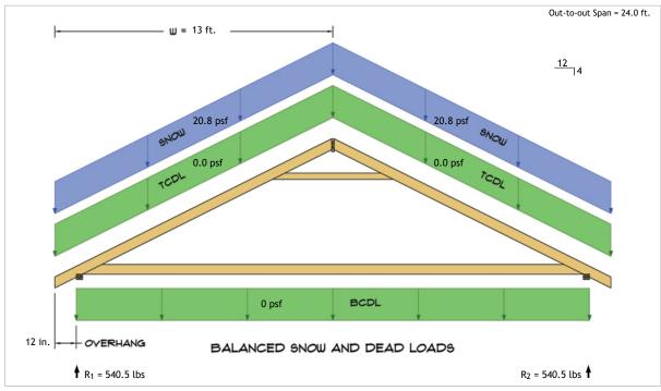
$R_1 = D + S = 0.0 \text{ lbs} + 540.5 \text{ lbs}$  $R_2 = D + S = 0.0 \text{ lbs} + 540.5 \text{ lbs}$
