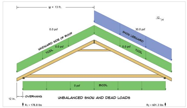
$R_1 = D + S = 0.0 \text{ lbs} + 178.8 \text{ lbs}$  $R_2 = D + S = 0.0 \text{ lbs} + 601.3 \text{ lbs}$
