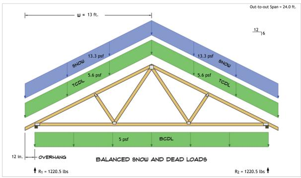
$$\begin{split} R_1 &= D + S = 530.7 \text{ lbs} + 689.8 \text{ lbs} \\ R_2 &= D + S = 530.7 \text{ lbs} + 689.8 \text{ lbs} \end{split}$$
