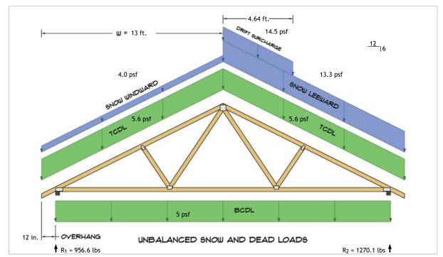
$R_1 = D + S = 530.7 \text{ lbs} + 425.9 \text{ lbs}$  $R_2 = D + S = 530.7 \text{ lbs} + 739.5 \text{ lbs}$
