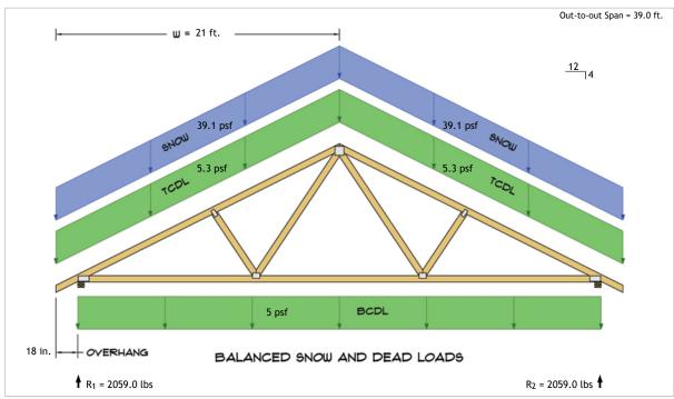
$$\begin{split} R_1 &= D + S = 416.4 \text{ lbs} + 1642.6 \text{ lbs} \\ R_2 &= D + S = 416.4 \text{ lbs} + 1642.6 \text{ lbs} \end{split}$$
