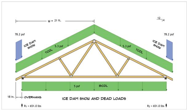
$R_1 = D + S = 416.4 \text{ lbs} + 234.7 \text{ lbs}$  $R_2 = D + S = 416.4 \text{ lbs} + 234.7 \text{ lbs}$
