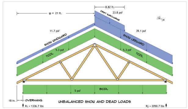
$R_1 = D + S = 416.4 \text{ lbs} + 920.4 \text{ lbs}$  $R_2 = D + S = 416.4 \text{ lbs} + 1634.3 \text{ lbs}$
