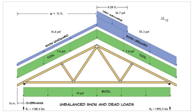
$R_1 = D + S = 395.3 \text{ lbs} + 793.1 \text{ lbs}$  $R_2 = D + S = 395.3 \text{ lbs} + 1600.1 \text{ lbs}$
