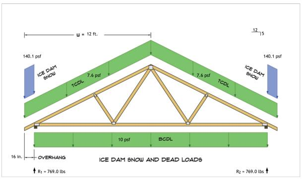
$$\begin{split} R_1 &= D + S = 395.3 \text{ lbs} + 373.7 \text{ lbs} \\ R_2 &= D + S = 395.3 \text{ lbs} + 373.7 \text{ lbs} \end{split}$$
