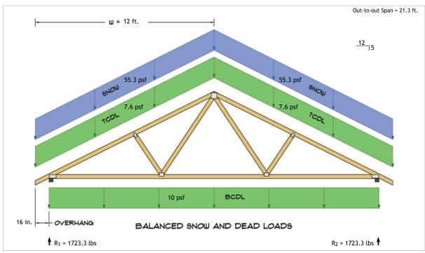
$$\begin{aligned} R_1 &= D + S = 395.3 \text{ lbs} + 1328.0 \text{ lbs} \\ R_2 &= D + S = 395.3 \text{ lbs} + 1328.0 \text{ lbs} \end{aligned}$$
