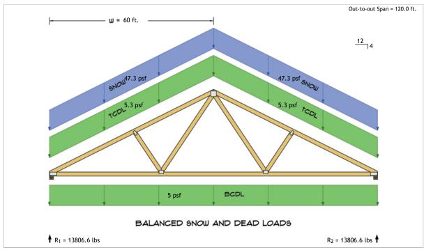
$R_1 = D + S = 2464.9 \text{ lbs} + 11341.6 \text{ lbs}$  $R_2 = D + S = 2464.9 \text{ lbs} + 11341.6 \text{ lbs}$
