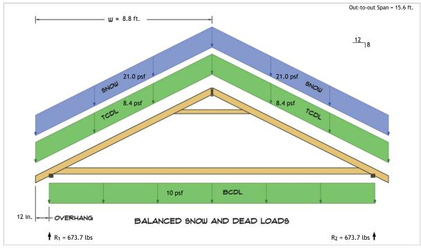
$R_1 = D + S = 304.1 \text{ lbs} + 369.6 \text{ lbs}$  $R_2 = D + S = 304.1 \text{ lbs} + 369.6 \text{ lbs}$
