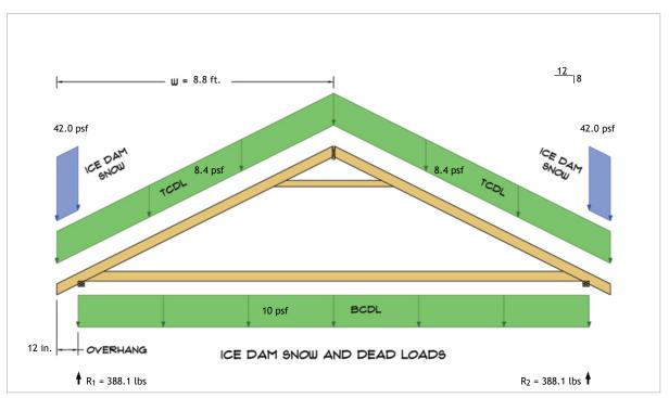
$R_1 = D + S = 304.1 \text{ lbs} + 84.0 \text{ lbs}$  $R_2 = D + S = 304.1 \text{ lbs} + 84.0 \text{ lbs}$
