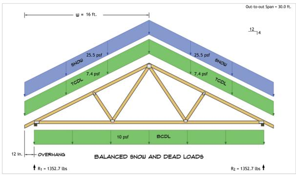
$$\begin{split} R_1 &= D + S = 536.1 \text{ lbs} + 816.6 \text{ lbs} \\ R_2 &= D + S = 536.1 \text{ lbs} + 816.6 \text{ lbs} \end{split}$$
