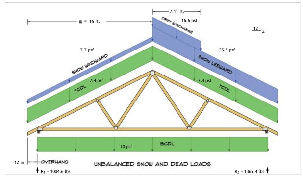
$R_1 = D + S = 536.1 \text{ lbs} + 468.5 \text{ lbs}$  $R_2 = D + S = 536.1 \text{ lbs} + 829.3 \text{ lbs}$
