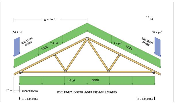
$R_1 = D + S = 536.1 \text{ lbs} + 108.9 \text{ lbs}$  $R_2 = D + S = 536.1 \text{ lbs} + 108.9 \text{ lbs}$
