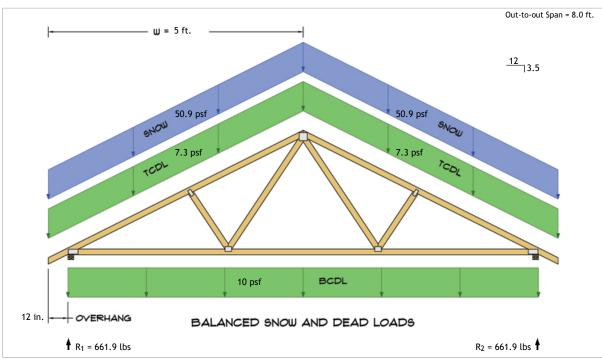
$$\begin{split} R_1 &= D + S = 152.9 \text{ lbs} + 509.0 \text{ lbs} \\ R_2 &= D + S = 152.9 \text{ lbs} + 509.0 \text{ lbs} \end{split}$$
