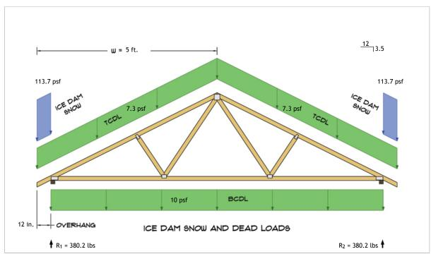
$R_1 = D + S = 152.9 \text{ lbs} + 227.3 \text{ lbs}$  $R_2 = D + S = 152.9 \text{ lbs} + 227.3 \text{ lbs}$
