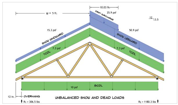
$R_1 = D + S = 152.9 \text{ lbs} + 153.6 \text{ lbs}$  $R_2 = D + S = 152.9 \text{ lbs} + 1027.4 \text{ lbs}$
