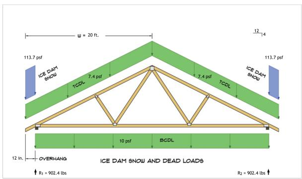
$R_1 = D + S = 675.1 \text{ lbs} + 227.3 \text{ lbs}$  $R_2 = D + S = 675.1 \text{ lbs} + 227.3 \text{ lbs}$
