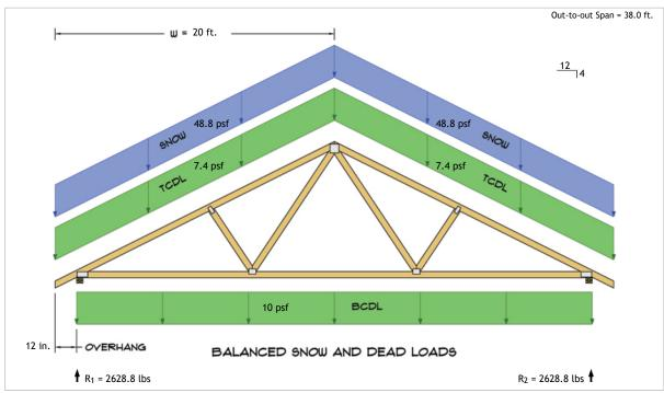
$\begin{aligned} R_1 &= D + S = 675.1 \text{ lbs} + 1953.7 \text{ lbs} \\ R_2 &= D + S = 675.1 \text{ lbs} + 1953.7 \text{ lbs} \end{aligned}$
