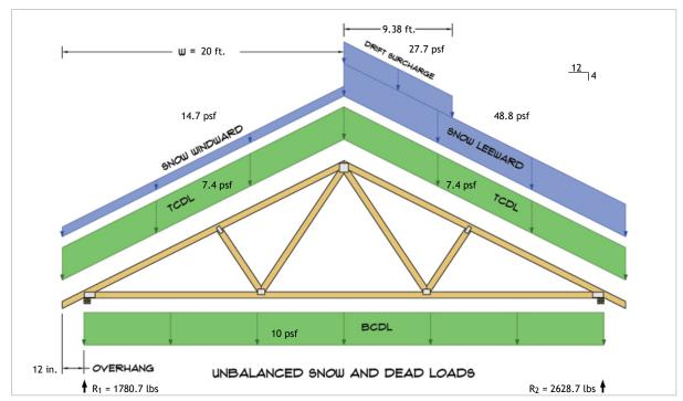
$R_1 = D + S = 675.1 \text{ lbs} + 1105.5 \text{ lbs}$  $R_2 = D + S = 675.1 \text{ lbs} + 1953.5 \text{ lbs}$
