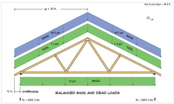
$\begin{aligned} R_1 &= D + S = 675.1 \text{ lbs} + 1980.2 \text{ lbs} \\ R_2 &= D + S = 675.1 \text{ lbs} + 1980.2 \text{ lbs} \end{aligned}$
