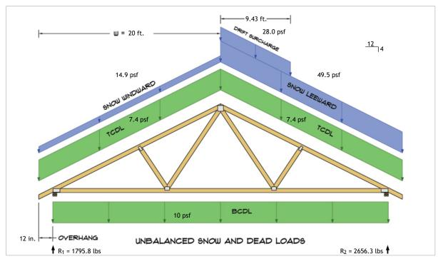
$R_1 = D + S = 675.1 \text{ lbs} + 1120.6 \text{ lbs}$  $R_2 = D + S = 675.1 \text{ lbs} + 1981.1 \text{ lbs}$
