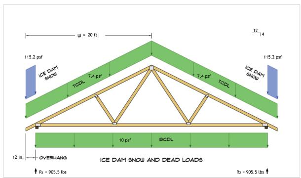
$R_1 = D + S = 675.1 \text{ lbs} + 230.4 \text{ lbs}$  $R_2 = D + S = 675.1 \text{ lbs} + 230.4 \text{ lbs}$
