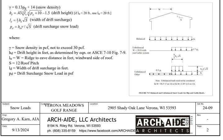
$$\begin{aligned} p_{\text{windward}} &= 0.3 \text{p}_{\text{s}} = (0.3)(37.4) = 11.2 \text{ psf} \\ p_{\text{leeward}} &= \text{p}_{\text{s}} = 37.4 \text{ psf} \end{aligned}$$
