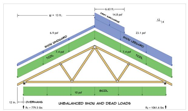
$R_1 = D + S = 431.8 \text{ lbs} + 347.7 \text{ lbs}$  $R_2 = D + S = 431.8 \text{ lbs} + 629.8 \text{ lbs}$
