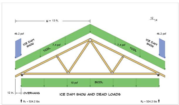
$R_1 = D + S = 431.8 \text{ lbs} + 92.4 \text{ lbs}$  $R_2 = D + S = 431.8 \text{ lbs} + 92.4 \text{ lbs}$
