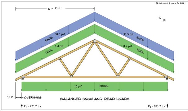
$R_1 = D + S = 305.8 \text{ lbs} + 667.3 \text{ lbs}$  $R_2 = D + S = 305.8 \text{ lbs} + 667.3 \text{ lbs}$
