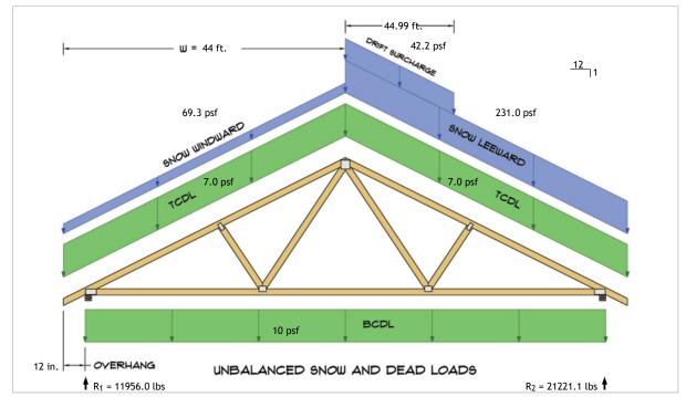
$R_1 = D + S = 1478.1 \text{ lbs} + 10477.9 \text{ lbs}$  $R_2 = D + S = 1478.1 \text{ lbs} + 19742.9 \text{ lbs}$
