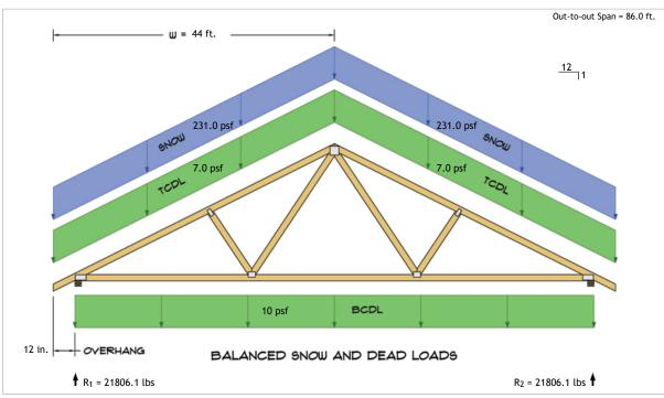
$$\begin{split} R_1 &= D + S = 1478.1 \text{ lbs} + 20328.0 \text{ lbs} \\ R_2 &= D + S = 1478.1 \text{ lbs} + 20328.0 \text{ lbs} \end{split}$$
