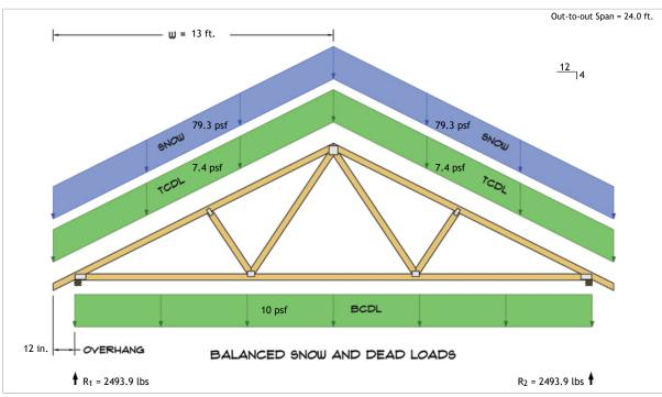
$\begin{aligned} R_1 &= D + S = 431.8 \text{ lbs} + 2062.1 \text{ lbs} \\ R_2 &= D + S = 431.8 \text{ lbs} + 2062.1 \text{ lbs} \end{aligned}$
