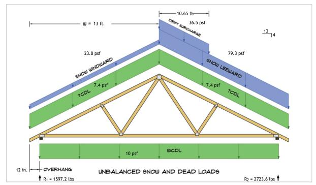
$R_1 = D + S = 431.8 \text{ lbs} + 1165.4 \text{ lbs}$  $R_2 = D + S = 431.8 \text{ lbs} + 2291.8 \text{ lbs}$
