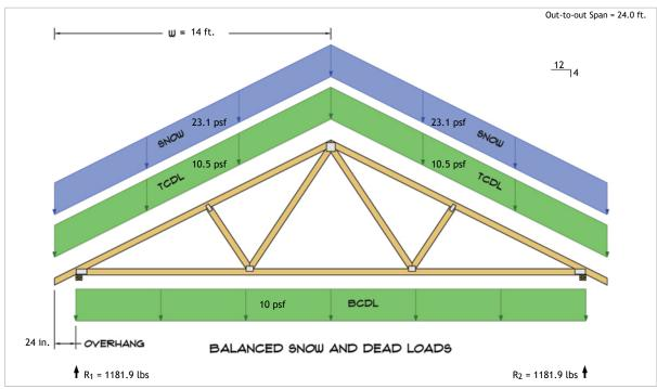
$$\begin{split} R_1 &= D + S = 535.1 \text{ lbs} + 646.8 \text{ lbs} \\ R_2 &= D + S = 535.1 \text{ lbs} + 646.8 \text{ lbs} \end{split}$$
