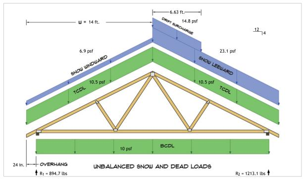
$R_1 = D + S = 535.1 \text{ lbs} + 359.5 \text{ lbs}$  $R_2 = D + S = 535.1 \text{ lbs} + 678.0 \text{ lbs}$
