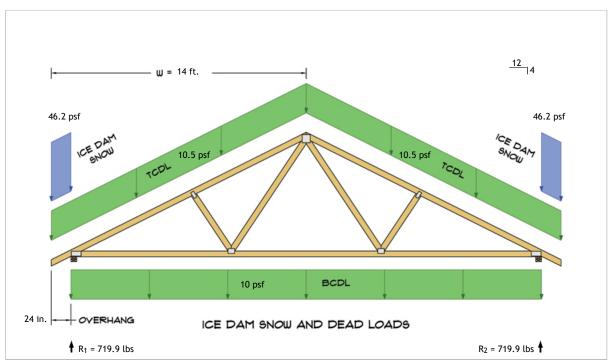
$R_1 = D + S = 535.1 \text{ lbs} + 184.8 \text{ lbs}$  $R_2 = D + S = 535.1 \text{ lbs} + 184.8 \text{ lbs}$
