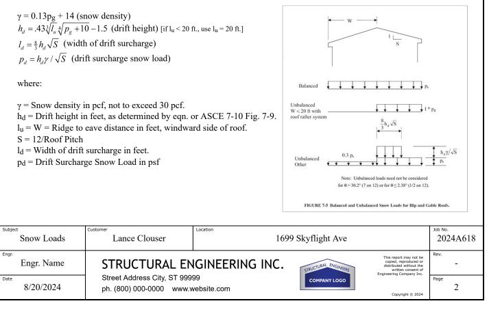
$$\begin{aligned} p_{\text{windward}} &= 0.3 \text{p}_{\text{s}} = (0.3)(33.1) = 9.9 \text{ psf} \\ p_{\text{leeward}} &= \text{p}_{\text{s}} = 33.1 \text{ psf} \end{aligned}$$
