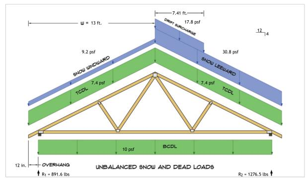
$\begin{aligned} R_1 &= D + S = 431.8 \text{ lbs} + 459.7 \text{ lbs} \\ R_2 &= D + S = 431.8 \text{ lbs} + 844.7 \text{ lbs} \end{aligned}$
