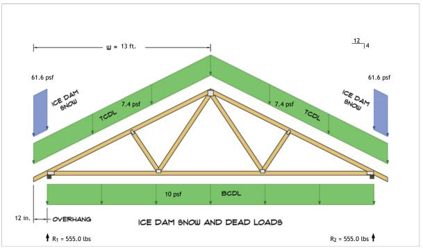
$R_1 = D + S = 431.8 \text{ lbs} + 123.2 \text{ lbs}$  $R_2 = D + S = 431.8 \text{ lbs} + 123.2 \text{ lbs}$
