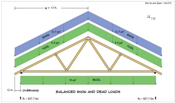
$R_1 = D + S = 497.4 \text{ lbs} + 330.3 \text{ lbs}$  $R_2 = D + S = 497.4 \text{ lbs} + 330.3 \text{ lbs}$
