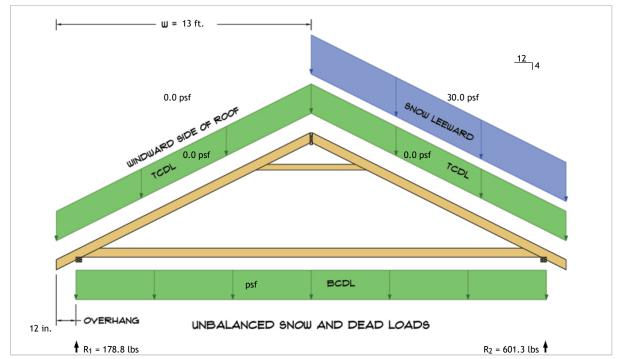
$\begin{aligned} R_1 &= D + S = 0.0 \text{ lbs} + 178.8 \text{ lbs} \\ R_2 &= D + S = 0.0 \text{ lbs} + 601.3 \text{ lbs} \end{aligned}$
