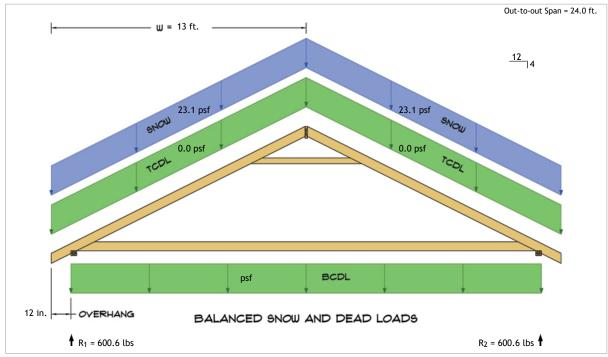
$R_1 = D + S = 0.0 \text{ lbs} + 600.6 \text{ lbs}$  $R_2 = D + S = 0.0 \text{ lbs} + 600.6 \text{ lbs}$
