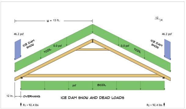
$\begin{aligned} R_1 &= D + S = 0.0 \text{ lbs} + 92.4 \text{ lbs} \\ R_2 &= D + S = 0.0 \text{ lbs} + 92.4 \text{ lbs} \end{aligned}$
