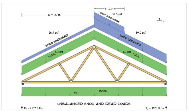
$R_1 = D + S = 130.7 \text{ lbs} + 2006.8 \text{ lbs}$  $R_2 = D + S = 130.7 \text{ lbs} + 3493.1 \text{ lbs}$
