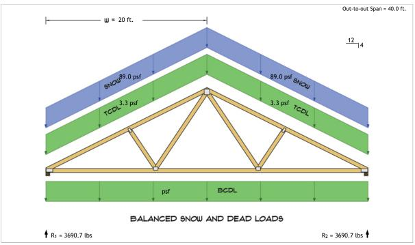
$R_1 = D + S = 130.7 \text{ lbs} + 3560.0 \text{ lbs}$  $R_2 = D + S = 130.7 \text{ lbs} + 3560.0 \text{ lbs}$
