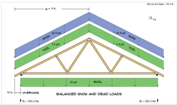
$$\begin{split} R_1 &= D + S = 199.9 \text{ lbs} + 323.4 \text{ lbs} \\ R_2 &= D + S = 199.9 \text{ lbs} + 323.4 \text{ lbs} \end{split}$$
