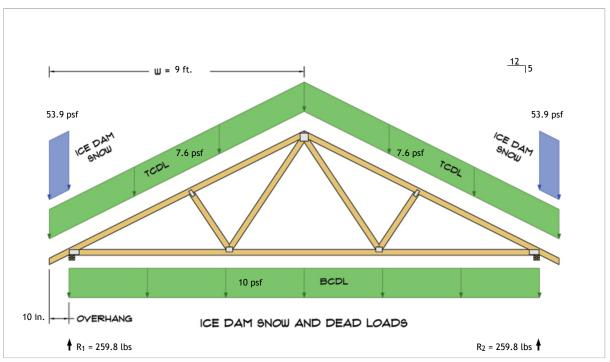
$$\begin{split} R_1 &= D + S = 199.9 \text{ lbs} + 59.9 \text{ lbs} \\ R_2 &= D + S = 199.9 \text{ lbs} + 59.9 \text{ lbs} \end{split}$$
