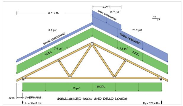
$R_1 = D + S = 199.9 \text{ lbs} + 194.9 \text{ lbs}$  $R_2 = D + S = 199.9 \text{ lbs} + 378.6 \text{ lbs}$
