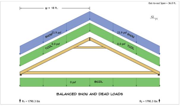
$R_1 = D + S = 0.0 \text{ lbs} + 1790.3 \text{ lbs}$  $R_2 = D + S = 0.0 \text{ lbs} + 1790.3 \text{ lbs}$
