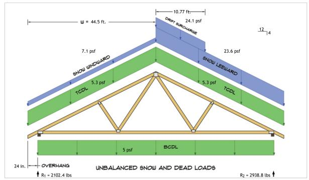
$R_1 = D + S = 894.1 \text{ lbs} + 1208.3 \text{ lbs}$  $R_2 = D + S = 894.1 \text{ lbs} + 2044.7 \text{ lbs}$
