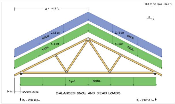
$\begin{aligned} R_1 &= D + S = 894.1 \text{ lbs} + 2102.9 \text{ lbs} \\ R_2 &= D + S = 894.1 \text{ lbs} + 2102.9 \text{ lbs} \end{aligned}$
