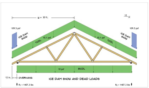
$R_1 = D + S = 1188.3 \text{ lbs} + 219.0 \text{ lbs}$  $R_2 = D + S = 1188.3 \text{ lbs} + 219.0 \text{ lbs}$
