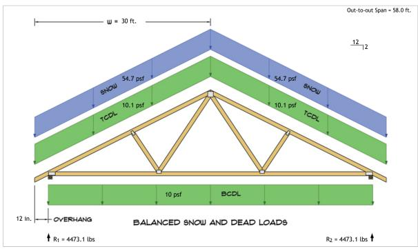
$$\begin{split} R_1 &= D + S = 1188.3 \text{ lbs} + 3284.8 \text{ lbs} \\ R_2 &= D + S = 1188.3 \text{ lbs} + 3284.8 \text{ lbs} \end{split}$$
