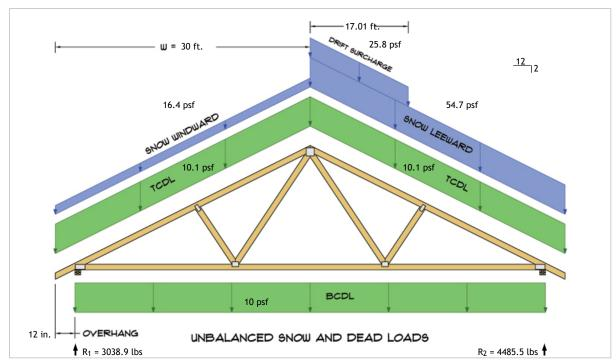
$R_1 = D + S = 1188.3 \text{ lbs} + 1850.6 \text{ lbs}$  $R_2 = D + S = 1188.3 \text{ lbs} + 3297.3 \text{ lbs}$
