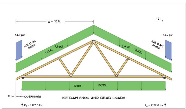
$R_1 = D + S = 1269.2 \text{ lbs} + 107.8 \text{ lbs}$  $R_2 = D + S = 1269.2 \text{ lbs} + 107.8 \text{ lbs}$
