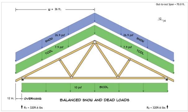
$$\begin{split} R_1 &= D + S = 1269.2 \text{ lbs} + 1940.4 \text{ lbs} \\ R_2 &= D + S = 1269.2 \text{ lbs} + 1940.4 \text{ lbs} \end{split}$$
