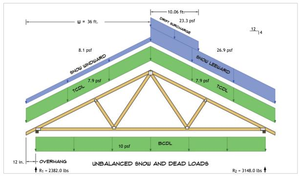
$R_1 = D + S = 1269.2 \text{ lbs} + 1112.8 \text{ lbs}$  $R_2 = D + S = 1269.2 \text{ lbs} + 1878.7 \text{ lbs}$
