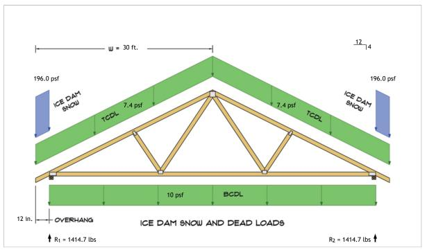
$$\begin{split} R_1 &= D + S = 1022.7 \text{ lbs} + 392.0 \text{ lbs} \\ R_2 &= D + S = 1022.7 \text{ lbs} + 392.0 \text{ lbs} \end{split}$$
