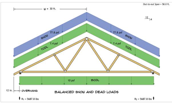
$$\begin{split} R_1 &= D + S = 1022.7 \text{ lbs} + 4665.1 \text{ lbs} \\ R_2 &= D + S = 1022.7 \text{ lbs} + 4665.1 \text{ lbs} \end{split}$$
