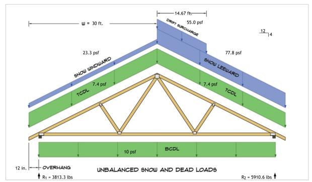
$R_1 = D + S = 1022.7 \text{ lbs} + 2790.6 \text{ lbs}$  $R_2 = D + S = 1022.7 \text{ lbs} + 4887.8 \text{ lbs}$
