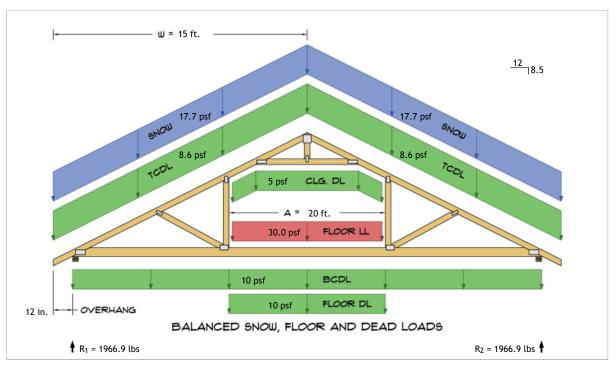
$$\begin{split} R_1 &= D + 0.75L + 0.75S = 837.3 \text{ lbs} + 600.0 \text{ lbs} + 529.6 \text{ lbs} \\ R_2 &= D + 0.75L + 0.75S = 837.3 \text{ lbs} + 600.0 \text{ lbs} + 529.6 \text{ lbs} \end{split}$$
