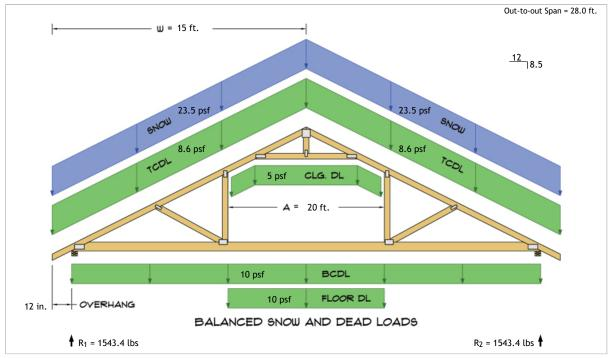
$R_1 = D + S = 837.3 \text{ lbs} + 706.1 \text{ lbs}$  $R_2 = D + S = 837.3 \text{ lbs} + 706.1 \text{ lbs}$
