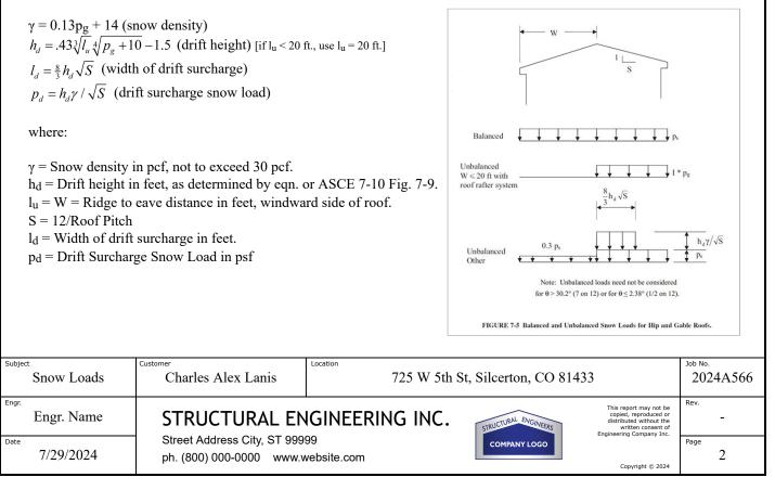
$$\begin{aligned} & \text{pwindward} = 0.3 \text{p}_{\text{s}} = (0.3)(62.6) = 18.8 \text{ psf} \\ & \text{pleeward} = \text{p}_{\text{s}} = 62.6 \text{ psf} \end{aligned}$$
