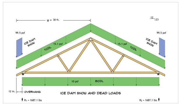
$\begin{aligned} R_1 &= D + S = 1488.0 \text{ lbs} + 199.1 \text{ lbs} \\ R_2 &= D + S = 1488.0 \text{ lbs} + 199.1 \text{ lbs} \end{aligned}$
