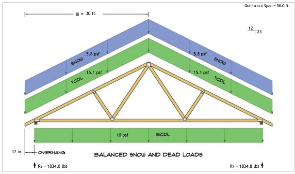
$R_1 = D + S = 1488.0 \text{ lbs} + 346.9 \text{ lbs}$  $R_2 = D + S = 1488.0 \text{ lbs} + 346.9 \text{ lbs}$
