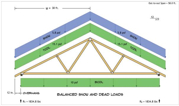
$R_1 = D + S = 1488.0 \text{ lbs} + 346.9 \text{ lbs}$  $R_2 = D + S = 1488.0 \text{ lbs} + 346.9 \text{ lbs}$
