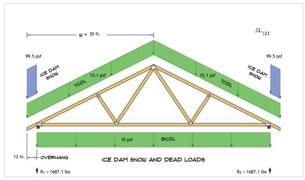
$R_1 = D + S = 1488.0 \text{ lbs} + 199.1 \text{ lbs}$  $R_2 = D + S = 1488.0 \text{ lbs} + 199.1 \text{ lbs}$
