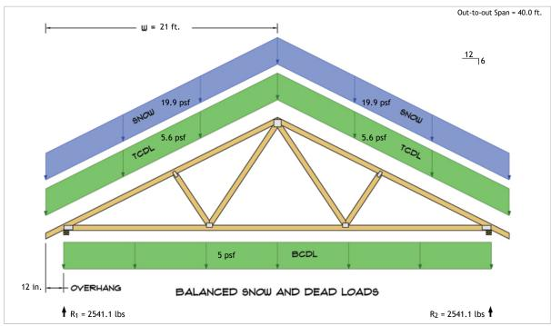
$\begin{aligned} R_1 &= D + S = 869.6 \text{ lbs} + 1671.5 \text{ lbs} \\ R_2 &= D + S = 869.6 \text{ lbs} + 1671.5 \text{ lbs} \end{aligned}$
