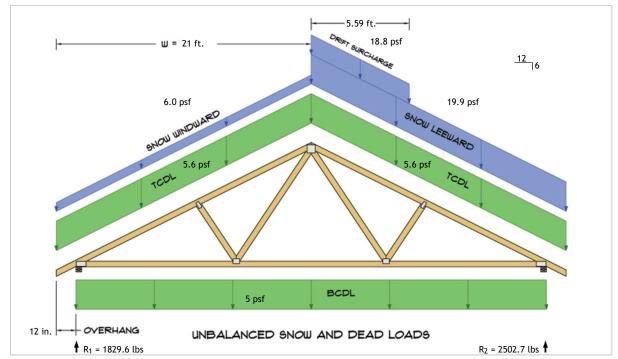
$R_1 = D + S = 869.6 \text{ lbs} + 960.0 \text{ lbs}$  $R_2 = D + S = 869.6 \text{ lbs} + 1633.1 \text{ lbs}$
