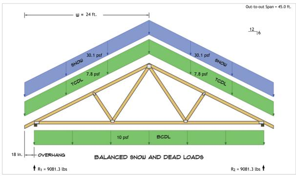
$$\begin{split} R_1 &= D + S = 3302.6 \text{ lbs} + 5778.6 \text{ lbs} \\ R_2 &= D + S = 3302.6 \text{ lbs} + 5778.6 \text{ lbs} \end{split}$$
