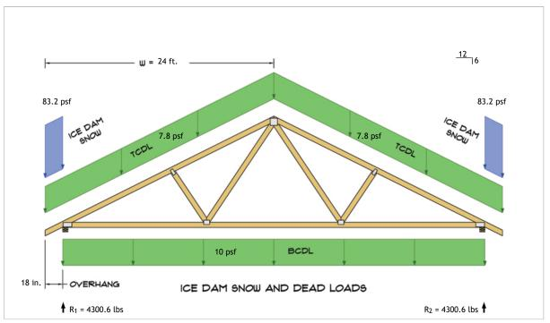
$$\begin{split} R_1 &= D + S = 3302.6 \text{ lbs} + 997.9 \text{ lbs} \\ R_2 &= D + S = 3302.6 \text{ lbs} + 997.9 \text{ lbs} \end{split}$$
