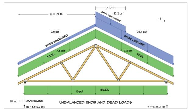
$R_1 = D + S = 3302.6 \text{ lbs} + 3513.6 \text{ lbs}$  $R_2 = D + S = 3302.6 \text{ lbs} + 6025.6 \text{ lbs}$
