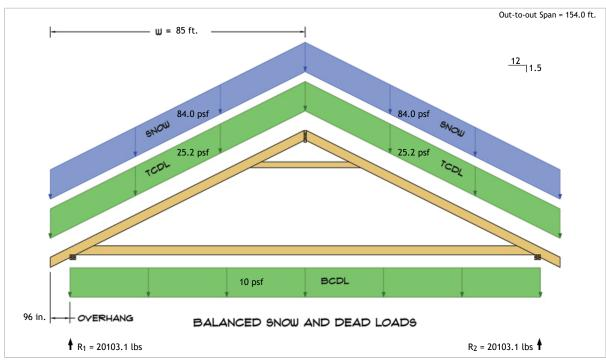
$$\begin{split} R_1 &= D + S = 5823.1 \text{ lbs} + 14280.0 \text{ lbs} \\ R_2 &= D + S = 5823.1 \text{ lbs} + 14280.0 \text{ lbs} \end{split}$$
