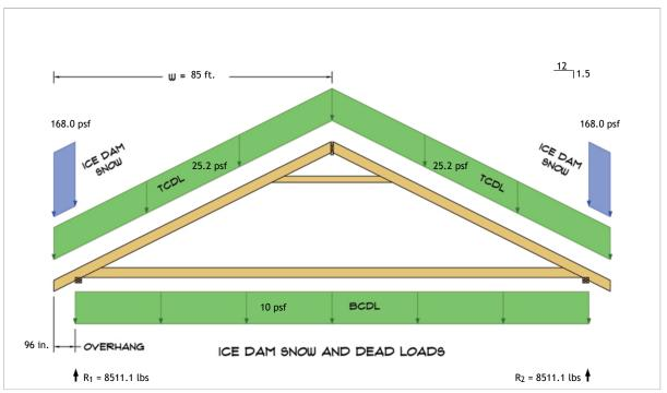
$$\begin{split} R_1 &= D + S = 5823.1 \text{ lbs} + 2688.0 \text{ lbs} \\ R_2 &= D + S = 5823.1 \text{ lbs} + 2688.0 \text{ lbs} \end{split}$$
