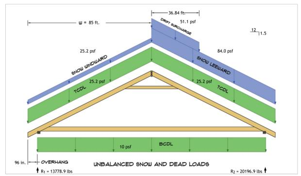
$R_1 = D + S = 5823.1 \text{ lbs} + 7955.8 \text{ lbs}$  $R_2 = D + S = 5823.1 \text{ lbs} + 14373.9 \text{ lbs}$
