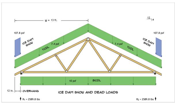
$R_1 = D + S = 1727.4 \text{ lbs} + 862.4 \text{ lbs}$  $R_2 = D + S = 1727.4 \text{ lbs} + 862.4 \text{ lbs}$
