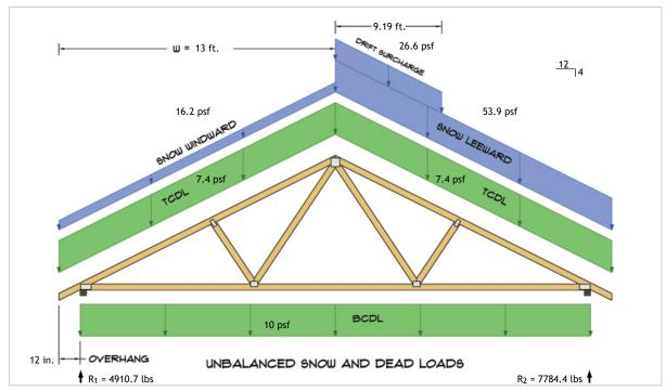
$R_1 = D + S = 1727.4 \text{ lbs} + 3183.3 \text{ lbs}$  $R_2 = D + S = 1727.4 \text{ lbs} + 6057.0 \text{ lbs}$
