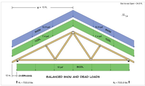
$$\begin{split} R_1 &= D + S = 1727.4 \text{ lbs} + 5605.6 \text{ lbs} \\ R_2 &= D + S = 1727.4 \text{ lbs} + 5605.6 \text{ lbs} \end{split}$$
