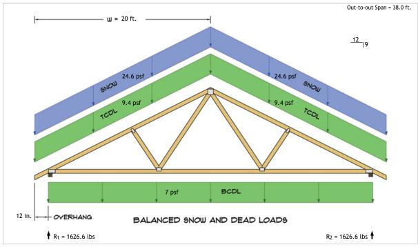
$R_1 = D + S = 641.0 \text{ lbs} + 985.6 \text{ lbs}$  $R_2 = D + S = 641.0 \text{ lbs} + 985.6 \text{ lbs}$
