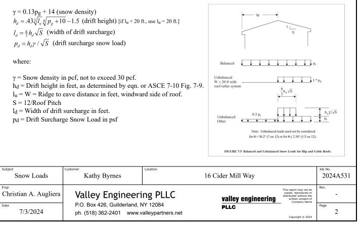
$$\begin{aligned} p_{\text{windward}} &= 0.3 \text{p}_{\text{s}} = (0.3)(34.7) = 10.4 \text{ psf} \\ p_{\text{leeward}} &= \text{p}_{\text{s}} = 34.7 \text{ psf} \end{aligned}$$
